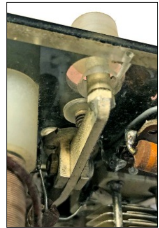
Detail view of the built-in miniature Morse key (right).
