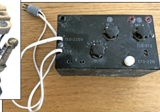
General view of the transmitter and power leads with plug to a power source (above).
