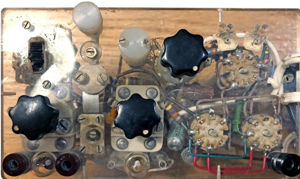
Top view of the transmitter with its (dark) top layer detached. Nearly all of the components of this transmitter, including valve holders, were mounted on the Plexiglas lower front panel.
